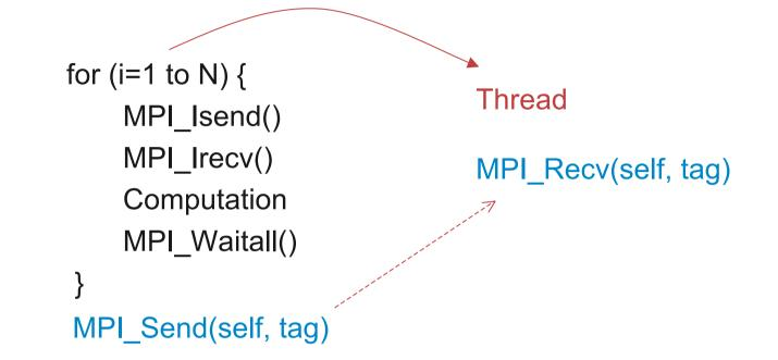
Measure time taken by the communication-computation loop with and without the thread
